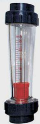
2. Rotameter's & Flowmeter's are crucial components of most processing systems. They are required to measure accurate amount of flow to be treated. In these environments, a pressure gauge needs to be reliable, accurate and easy to read to help prevent failure in everyday operations. Rota meter is manually calibrated flow measuring instrument with glass Indicators, whereas flowmeter is an electronic, electromagnetic or ultrasonic instrument.
