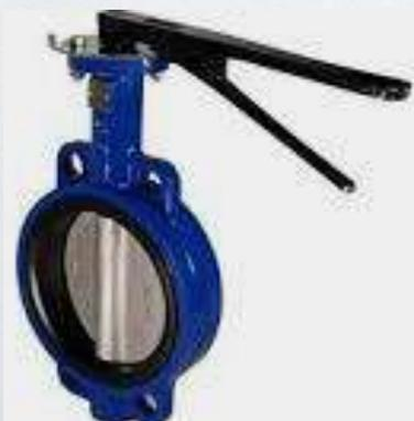
3. The **Butterfly valve** is **used** to regulate and control, throttle the flow. They are featured by a fast operation and low-pressure drop. To make an open position from the closed, it requires only a quarter turn. Wafer, lug, Single-Flange, Flange are the regular types of **butterfly valves**. These can be opened for checks and re used.
